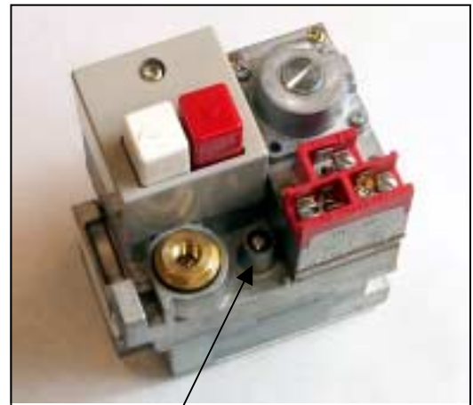
The pilot adjustment on the CE valve is here.
