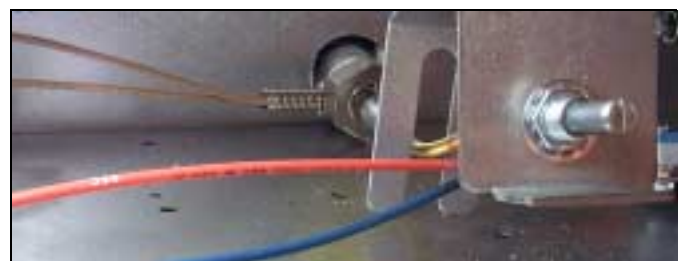
The flexible shaft on the G series thermostat must be removed to access the operating thermostat.
